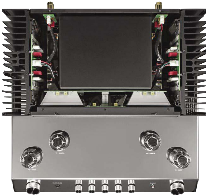
With top cover removed the screened mains transformer can be seen, with power amplifier boards mounted in heatsinks either side. Convection cooling only (no fan) with thermal cutout; ours ran just warm.
