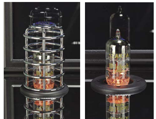
Safety covers over the valves lift off. The bright orange glow comes from underside LEDs, orange indicating warm up or overload.
